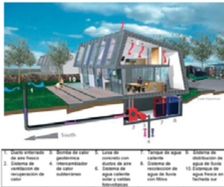
Imagen N°1: Elementos para la eficiencia energética en edificaciones. Fuente: Energy efficiency in buildings - Facts and trends, World Business Council for Sustainable Development, October (2007) .
